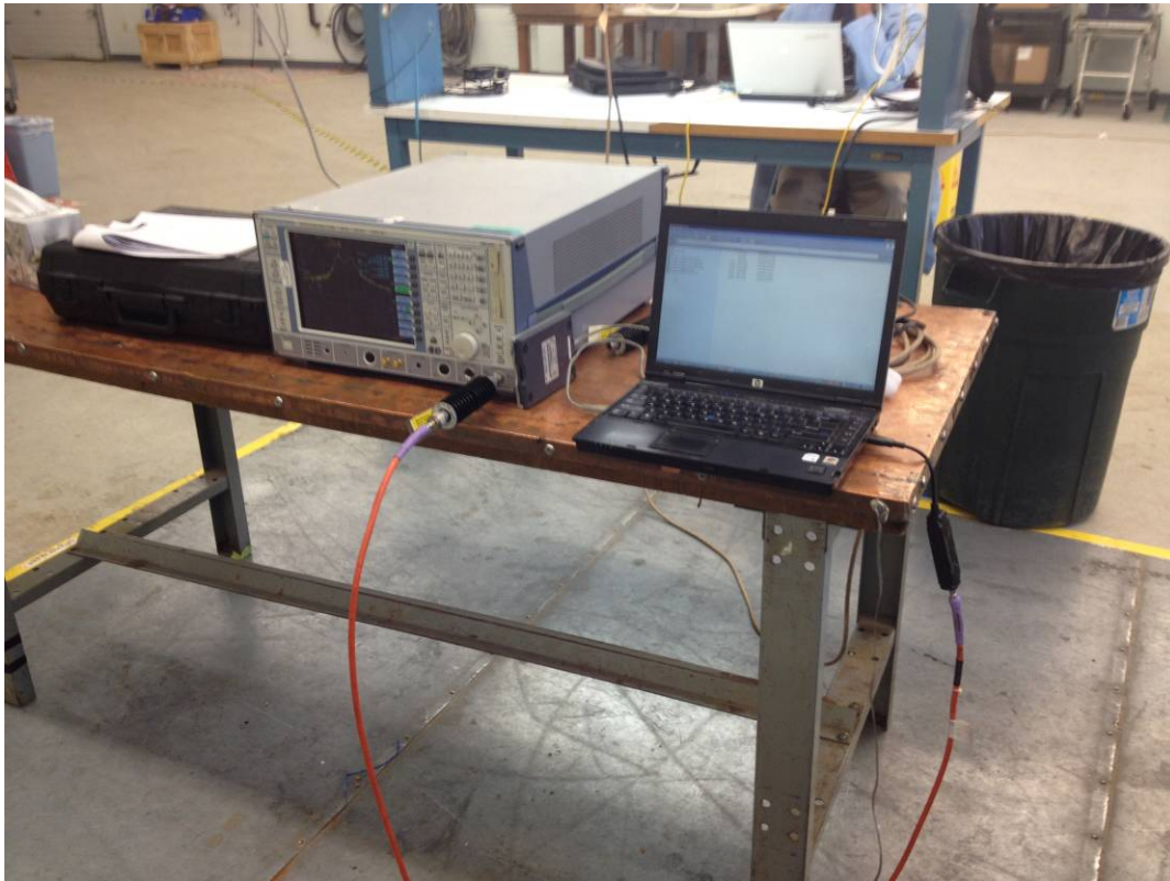
Antenna Port Conducted Test Setup
