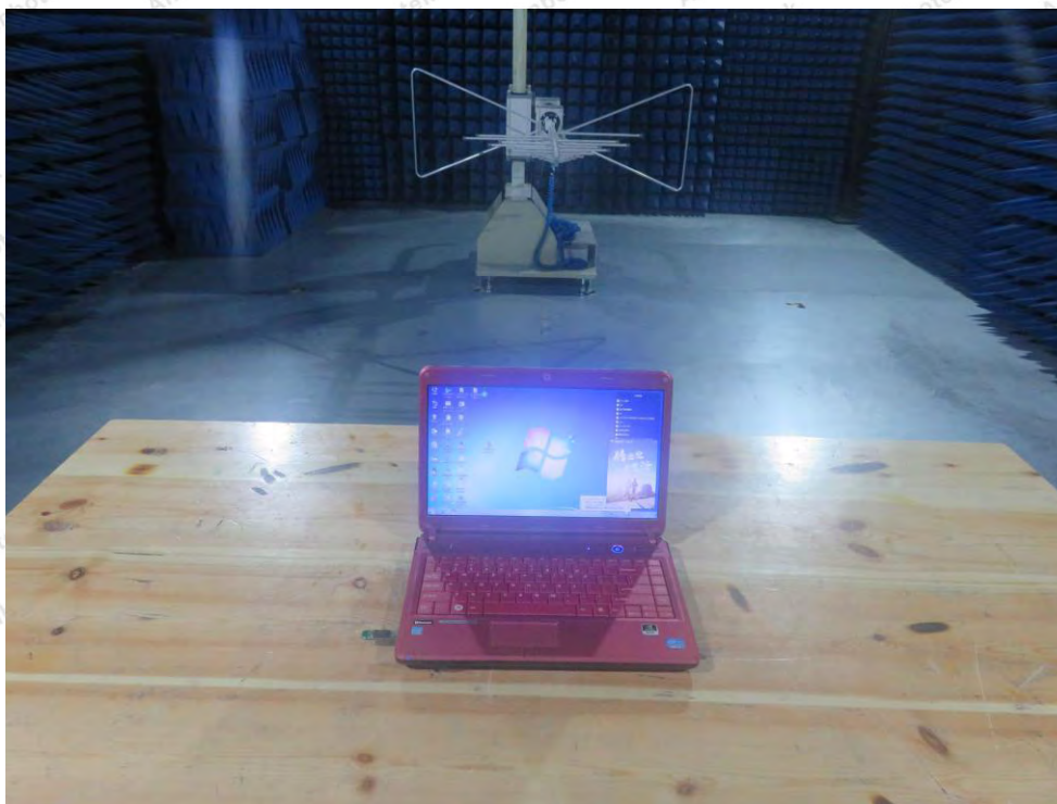
Photo of Radiation Emission Test
