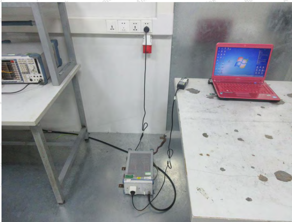
Photo of Conducted Emission Measurement
