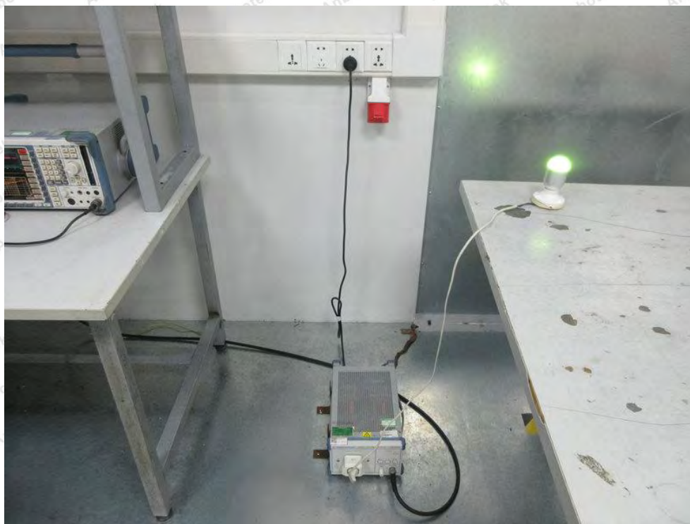
Photo of Conducted Emission Measurement
