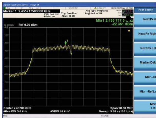
(802.11n20) PSD plot on channel 11
