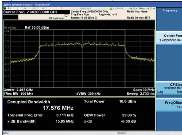
(802.11n20) 6dB Bandwidth plot on channel 11
