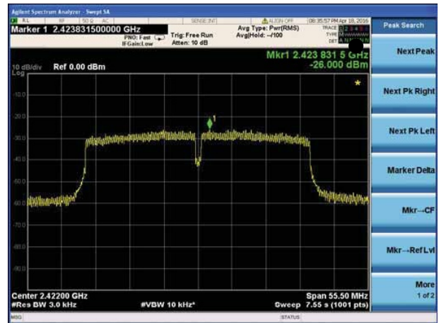
(802.11n40) PSD plot on channel 6
