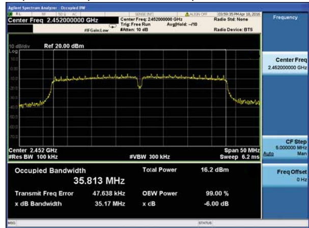
(802.11n40) 6dB Bandwidth plot on channel 9
