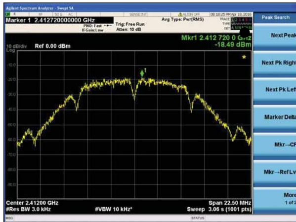
(802.11b) PSD plot on channel 6
