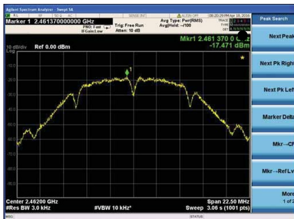
(802.11b) PSD plot on channel 11
