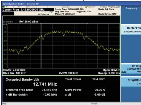
(802.11b) 6dB Bandwidth plot on channel 11
