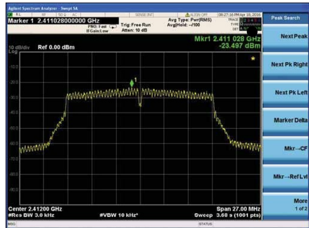
(802.11g) PSD plot on channel 6
