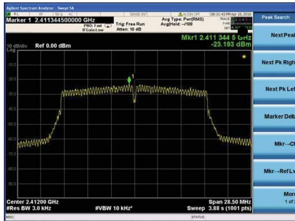
(802.11n20) PSD plot on channel 6
