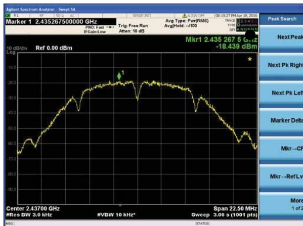
(802.11b) PSD plot on channel 11
