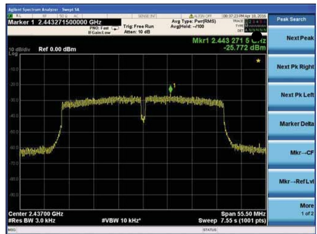
(802.11n40) PSD plot on channel 9
