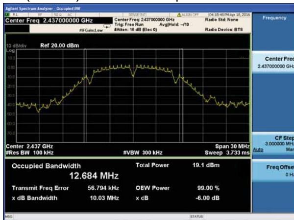
(802.11b) 6dB Bandwidth plot on channel 6
