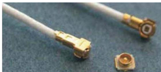
Figure 17: The profile of the I-PEX connector
