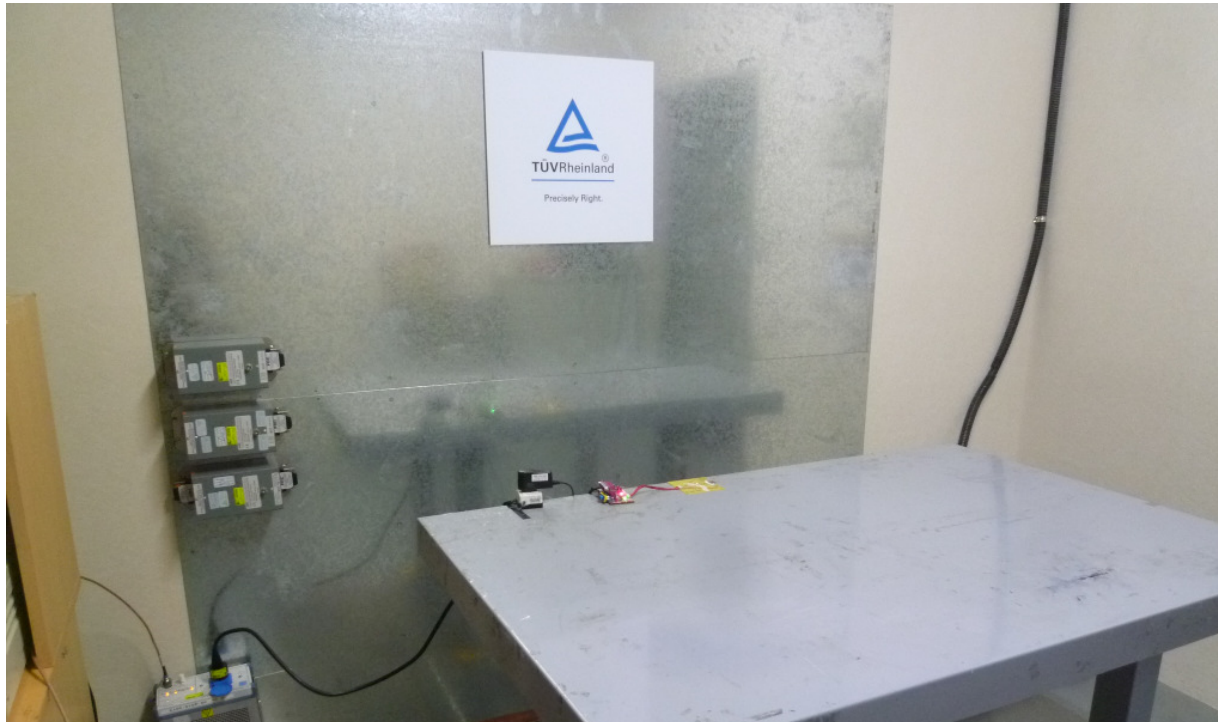
Photograph 9: Set-up for Mains Conducted testing Front
