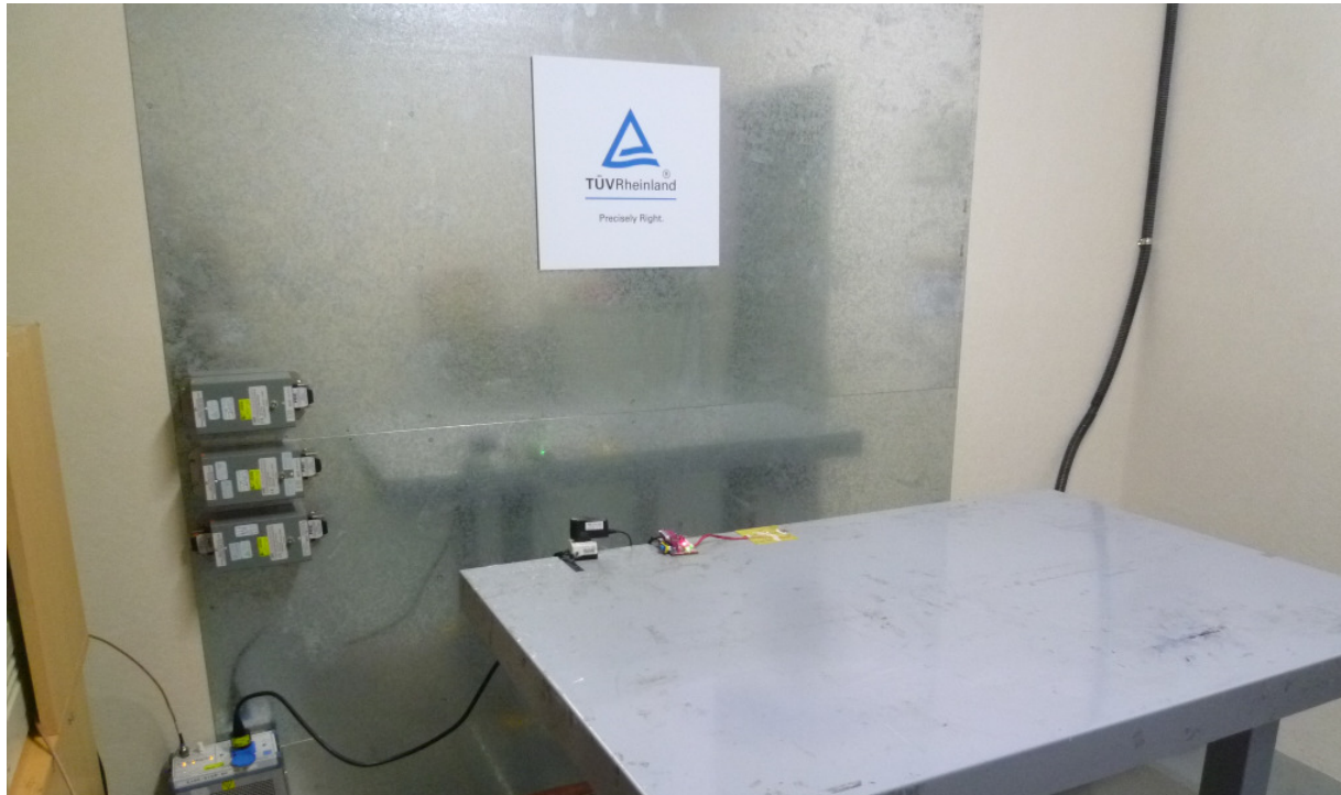
Photograph 9: Set-up for Mains Conducted testing Front
