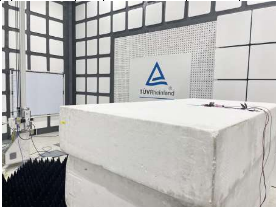
Photograph 6: Test Setup for Spurious Emissions (Back View 4)
