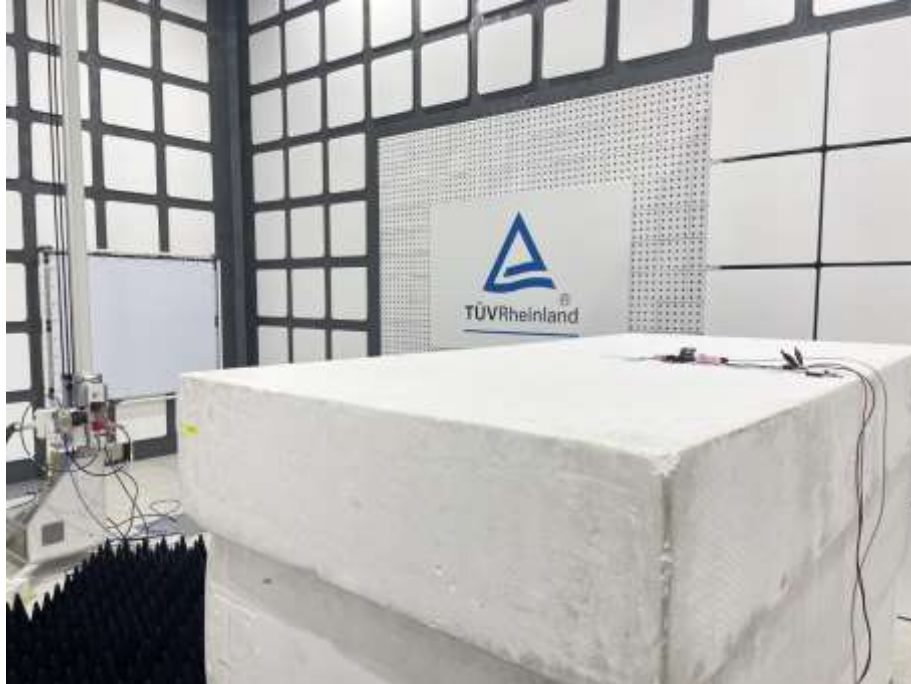
Photograph 5: Test Setup for Spurious Emissions (Back View 3)
