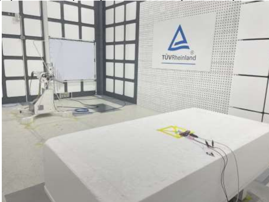
Photograph 4: Test Setup for Spurious Emissions (Back View 2)
