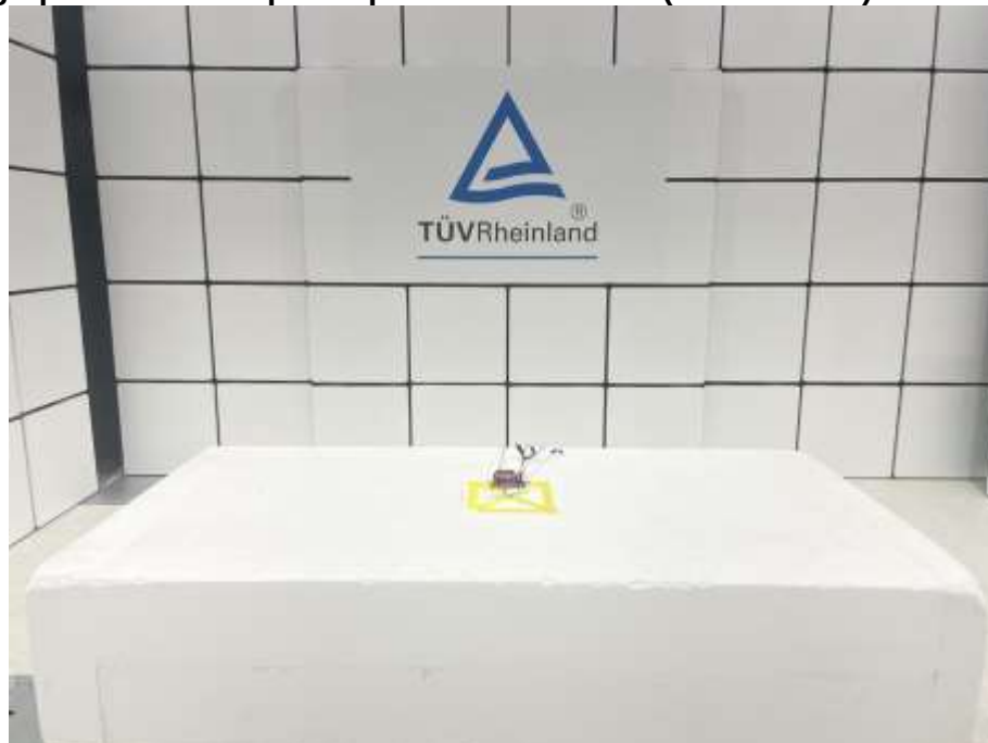
Photograph 2: Test Setup for Spurious Emissions (Front View 2)
