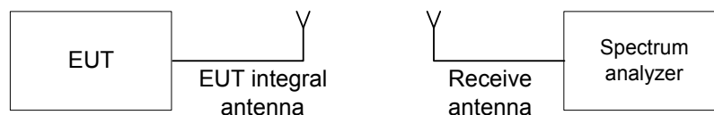
Figure 7.1.1 Setup for transmitter shut down test
