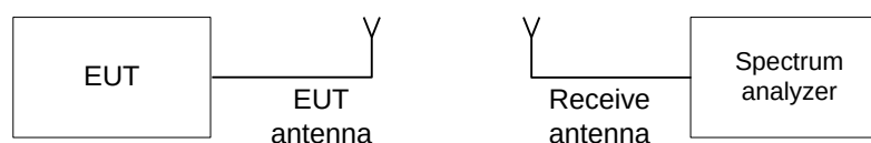
Figure 7.4.1 Occupied bandwidth test setup
