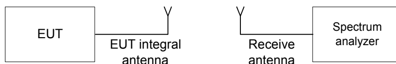
Figure 7.1.1 Setup for transmitter shut down test
