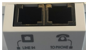
Figure 12: The PSTN Phone Sockets
