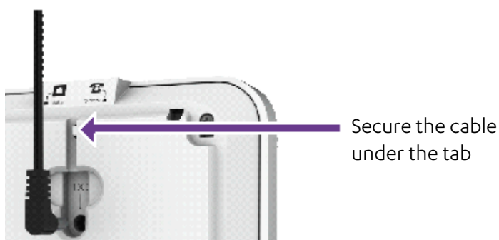
Figure 8: Connecting the Power Adapter's Cable
