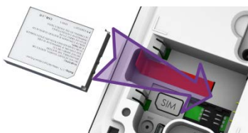
Figure 6: Inserting Backup Battery
