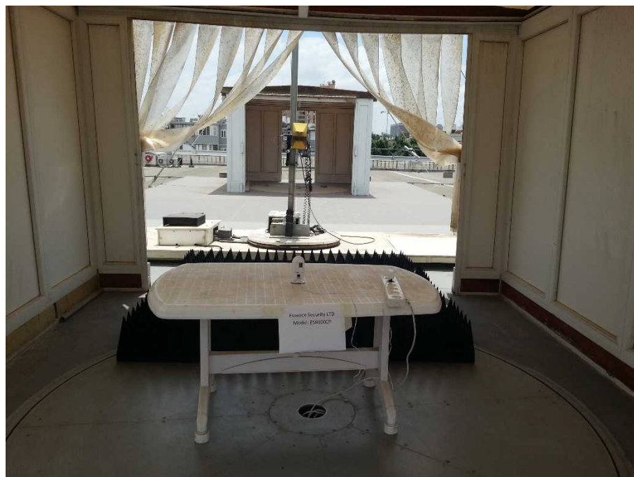
Figure 5. Radiated Emission Test
