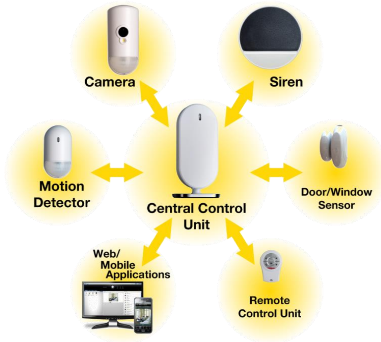
Figure 2: We.R™ Home Area Network Components
