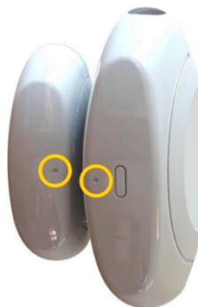
Figure 82: Dot Alignment of the Magnetic Sensor Units
