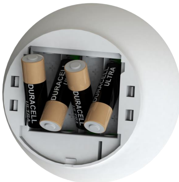
Figure 97: Inserting the Batteries into the Siren
