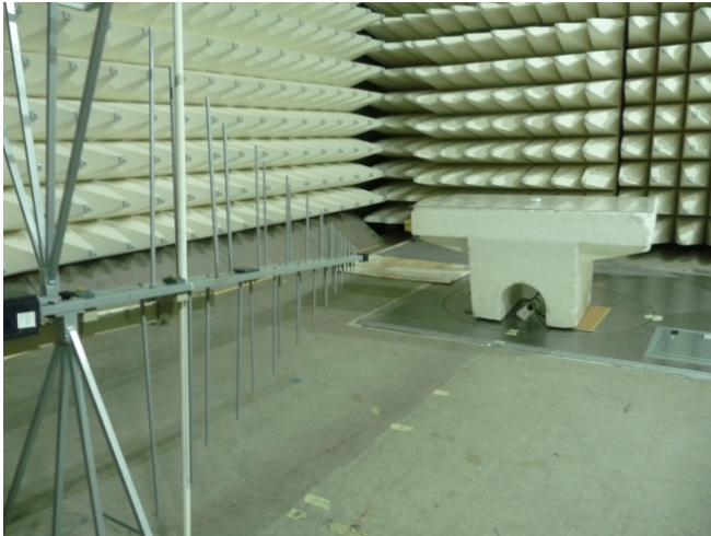
Photograph 8.1.1 Setup for radiated emission measurements
