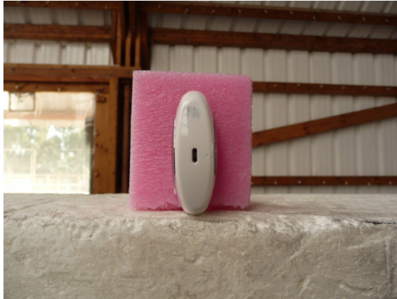
Photograph 6.4.2 EUT in Y-axis orthogonal position
