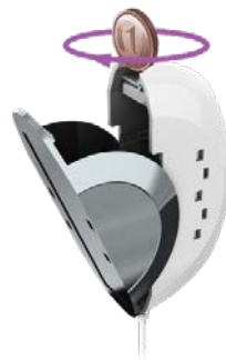
Figure 43: Releasing the Transmitter Base
