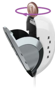
Figure 39: Releasing the Transmitter
