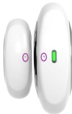
Figure 26: Dot Alignment of the Door/Window Sensor
