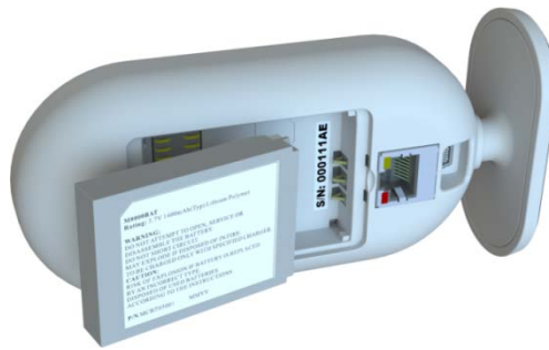
Figure 4: Insert Backup Battery
