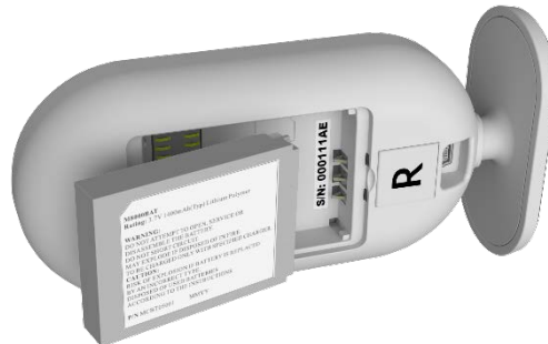
Figure 46: Insert Backup Battery
