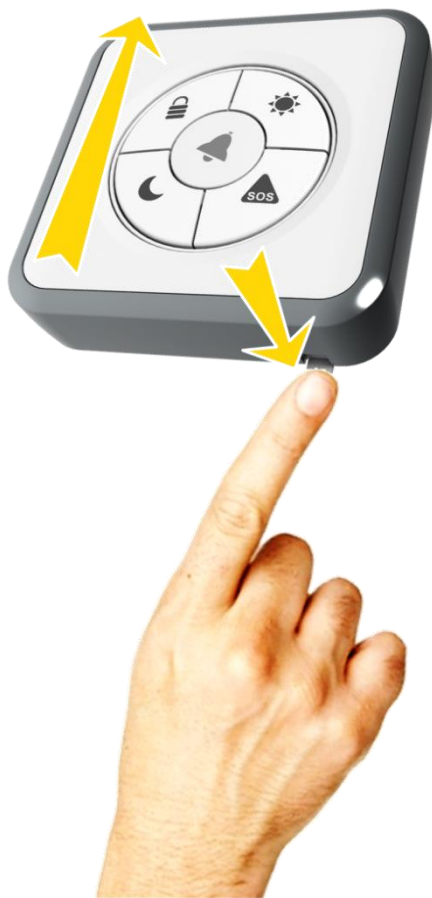
Figure 207: Dismounting the Tag Reader
