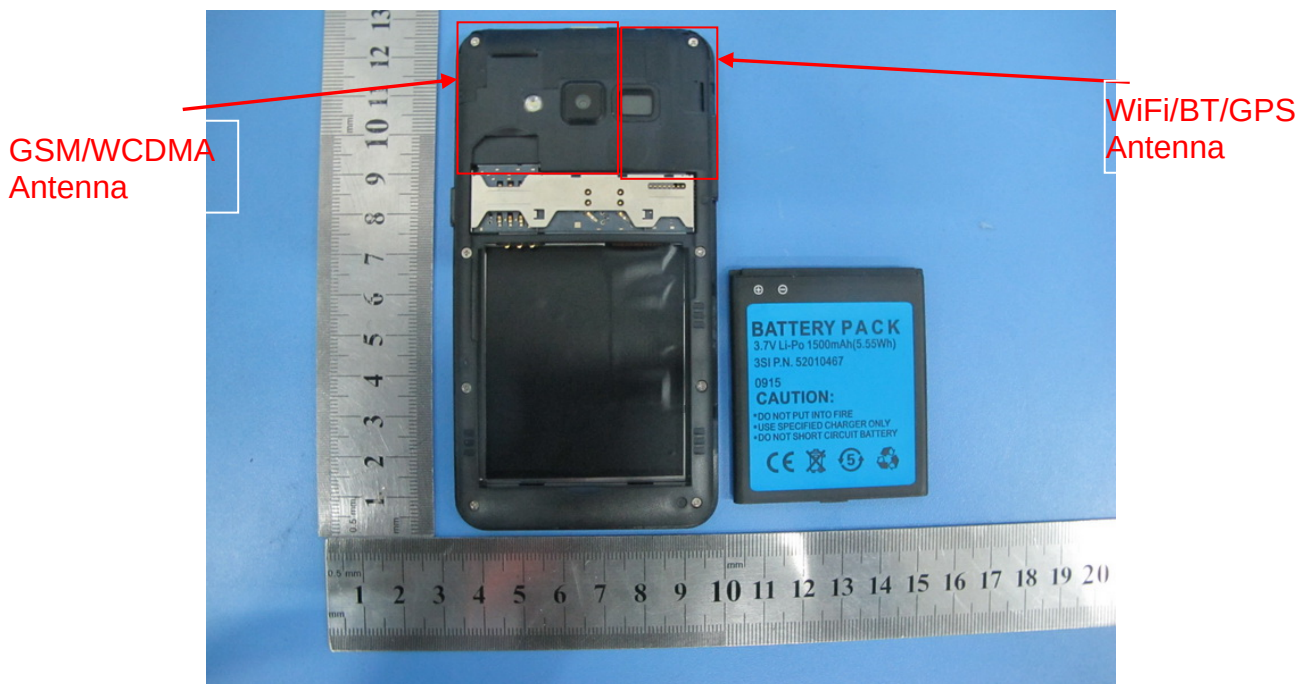
Photo 7 Internal of EUT
