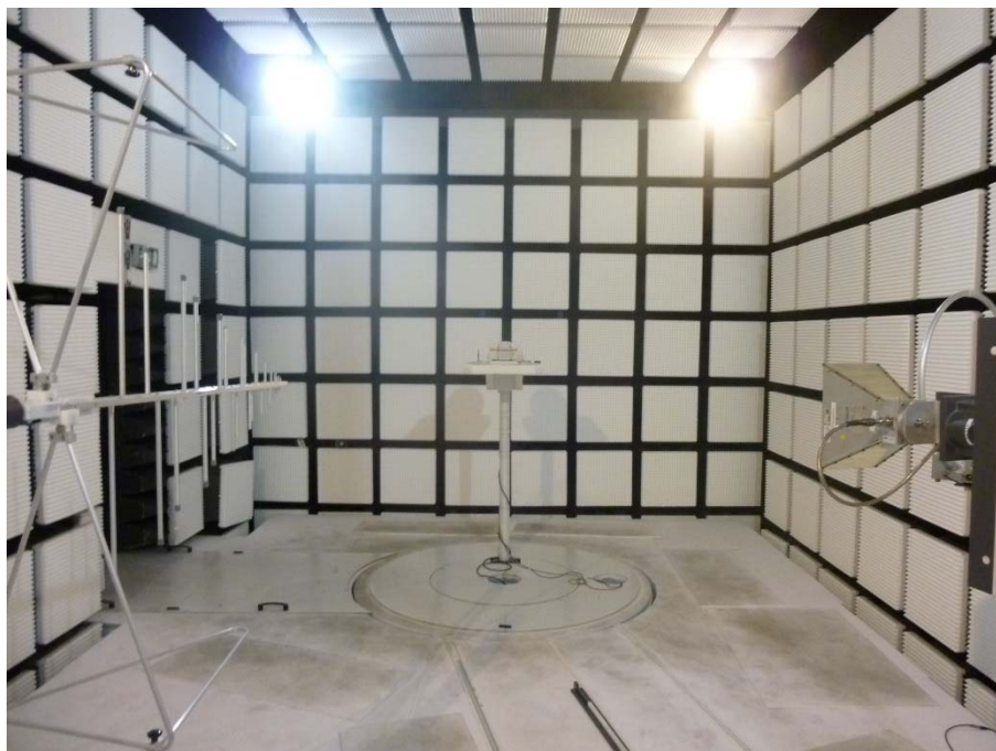
Photo 6: EUT at the anechoic chamber
