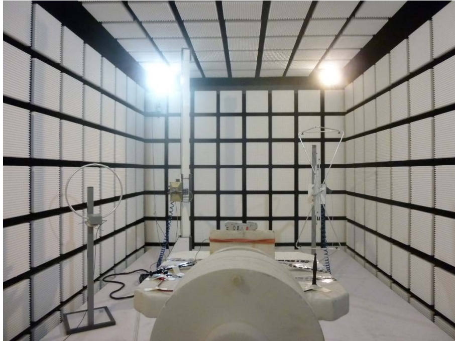
Photo 3: EUT at the anechoic chamber
