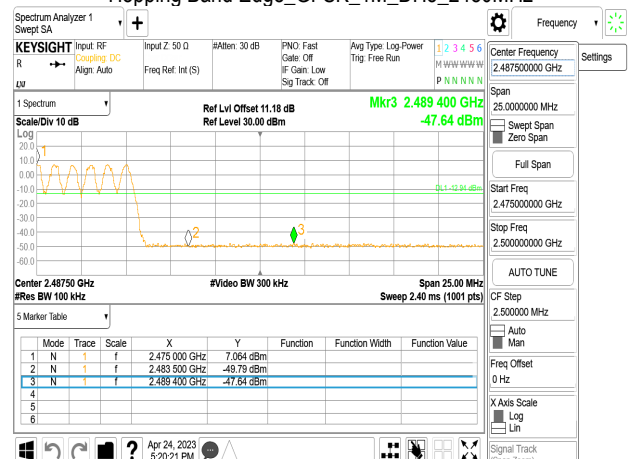
Hopping Band Edge_GFSK_1M_DH5_2480MHz
