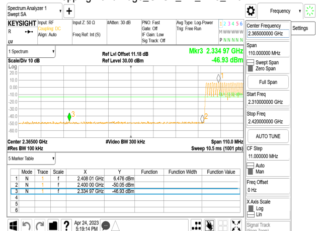
Hopping Band Edge_GFSK_1M_DH5_2480MHz
