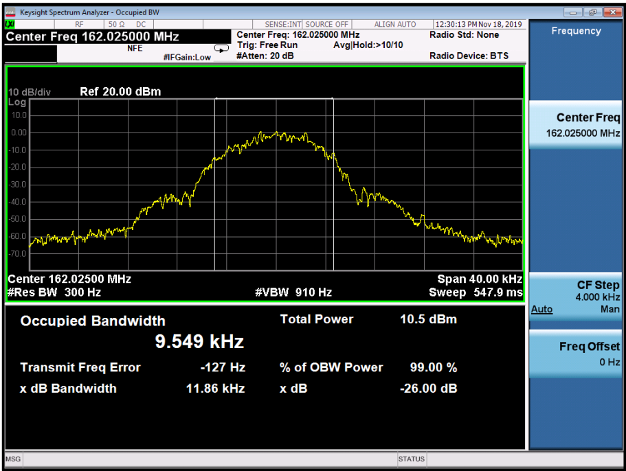
Figure 2 - 162.025 MHz Occupied Bandwidth
