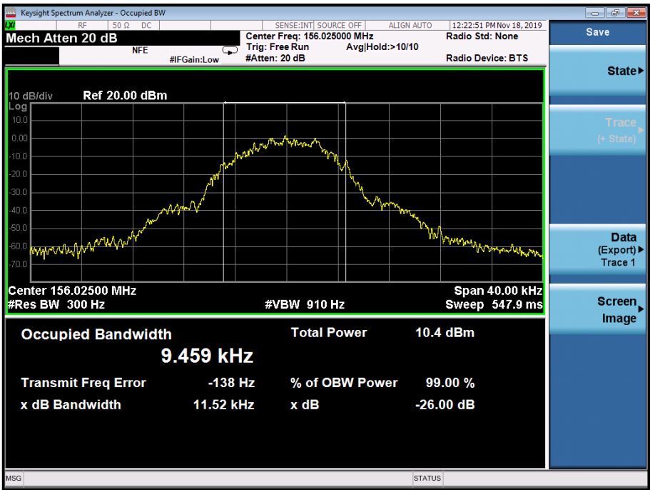
Figure 1 - 156.025 MHz Occupied Bandwidth
