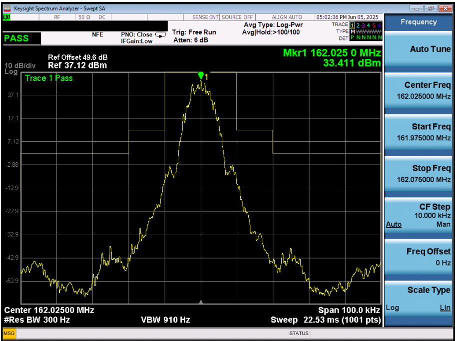
Figure 5 – Tx2, 156.025 MHz - Transmitter Spectrum Mask
