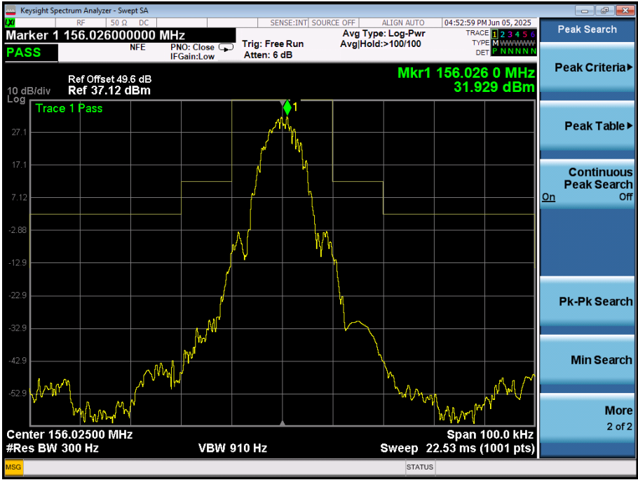
Figure 3 – Tx1, 156.025 MHz - Transmitter Spectrum Mask
