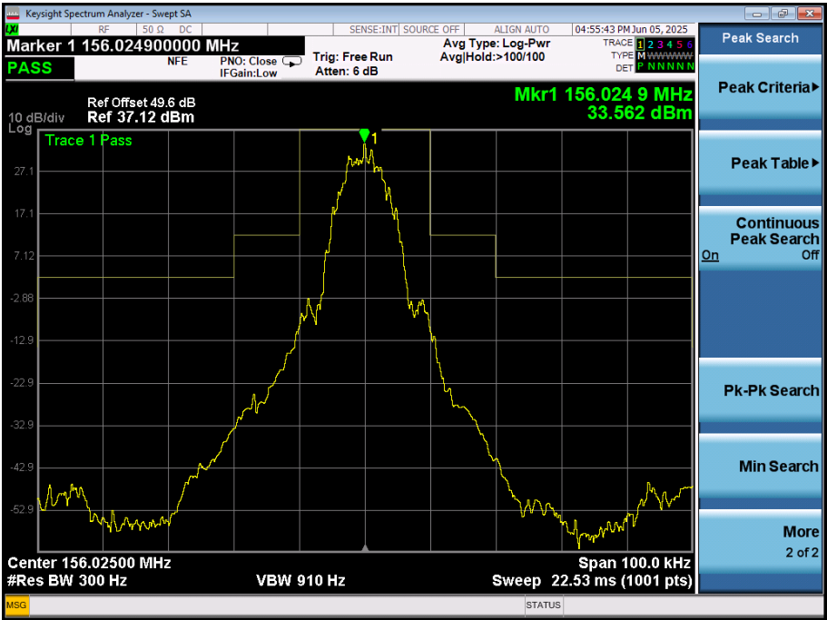
Figure 5 – Tx2, 156.025 MHz - Transmitter Spectrum Mask
