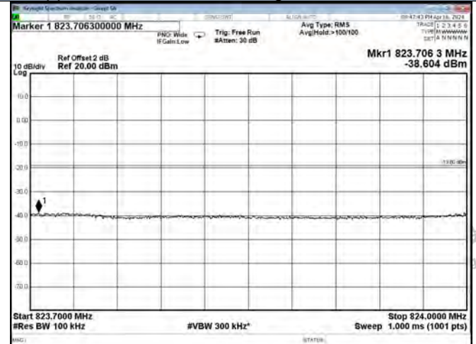
Cellular Band UL-LTE Left Side AGC+10dB
