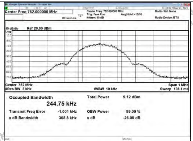
GSM-Upper 700 Band DL Output
