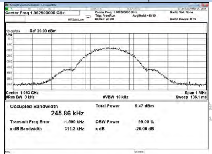
GSM-PCS Band DL Output
