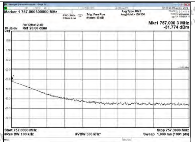
Upper 700 Band DL-GSM Right Side AGC+10dB
