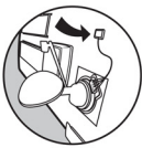
Option 1: Using existing cable entry point.
