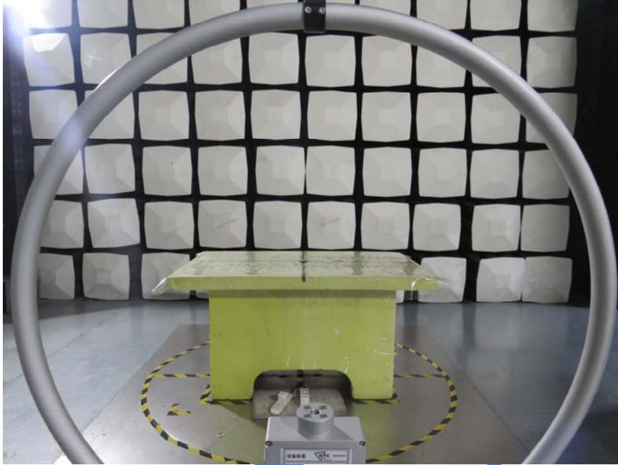
Test Photo Radiated emission (Below 30MHz)
