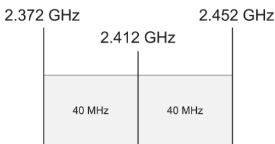
Figure 5–1 Channel, 80 MHz Wide Frequency Band
