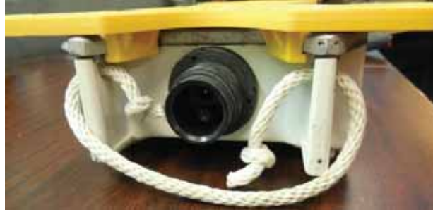
Figure 2-15 Anchor Plate at WRU Geophone End
