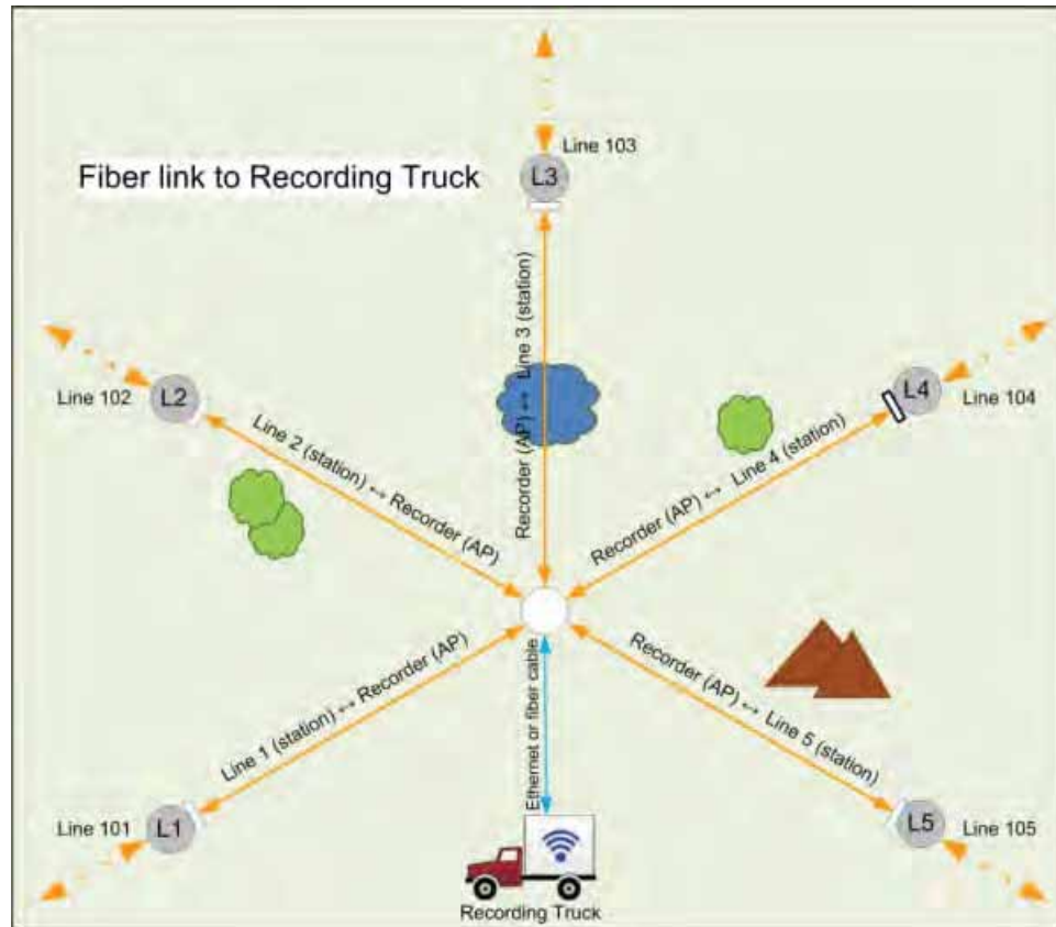
Figure 5–26 Connecting the Recording Truck with Fiber
