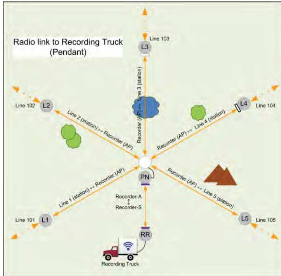
Figure 5–27 Connecting the Recording Truck with a Pendant Radio Link
