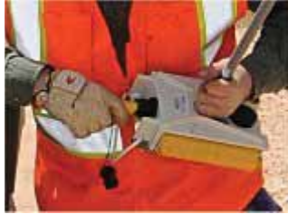
Figure 2-7 Installing the Geophone
