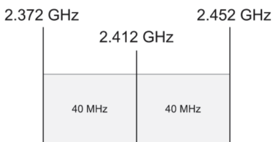
Figure 5–1 Channel, 80 MHz Wide Frequency Band
