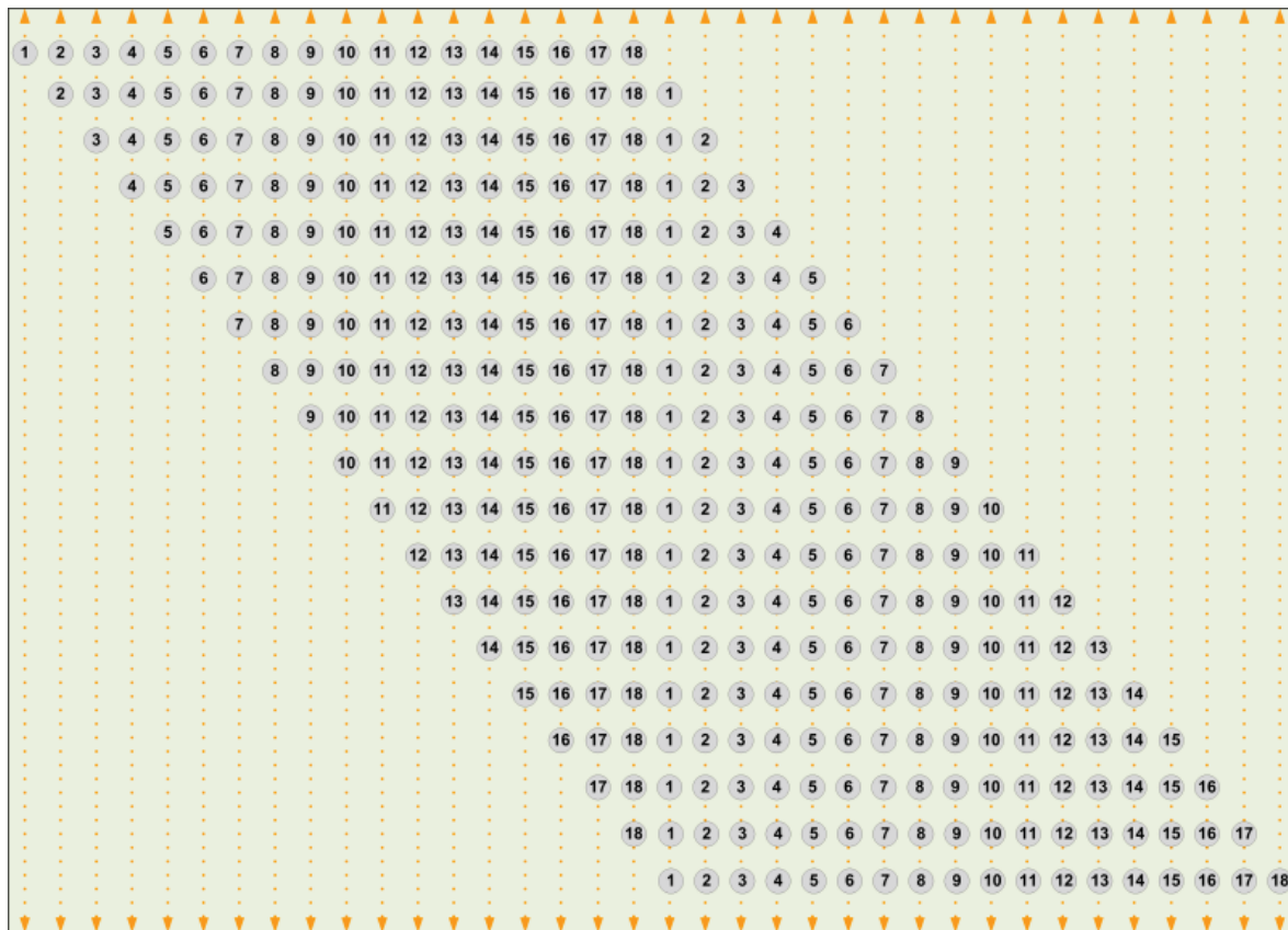
Figure 4–23 Rolling Scheme, 18 Total Poles Example
