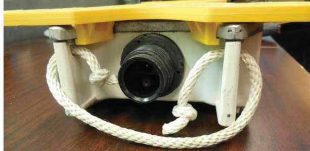
Figure 2-15 Anchor Plate at WRU Geophone End
