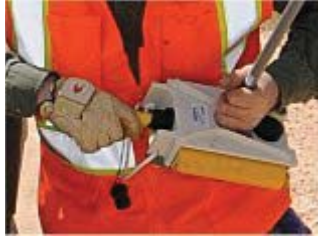
Figure 2-7 Installing the Geophone
