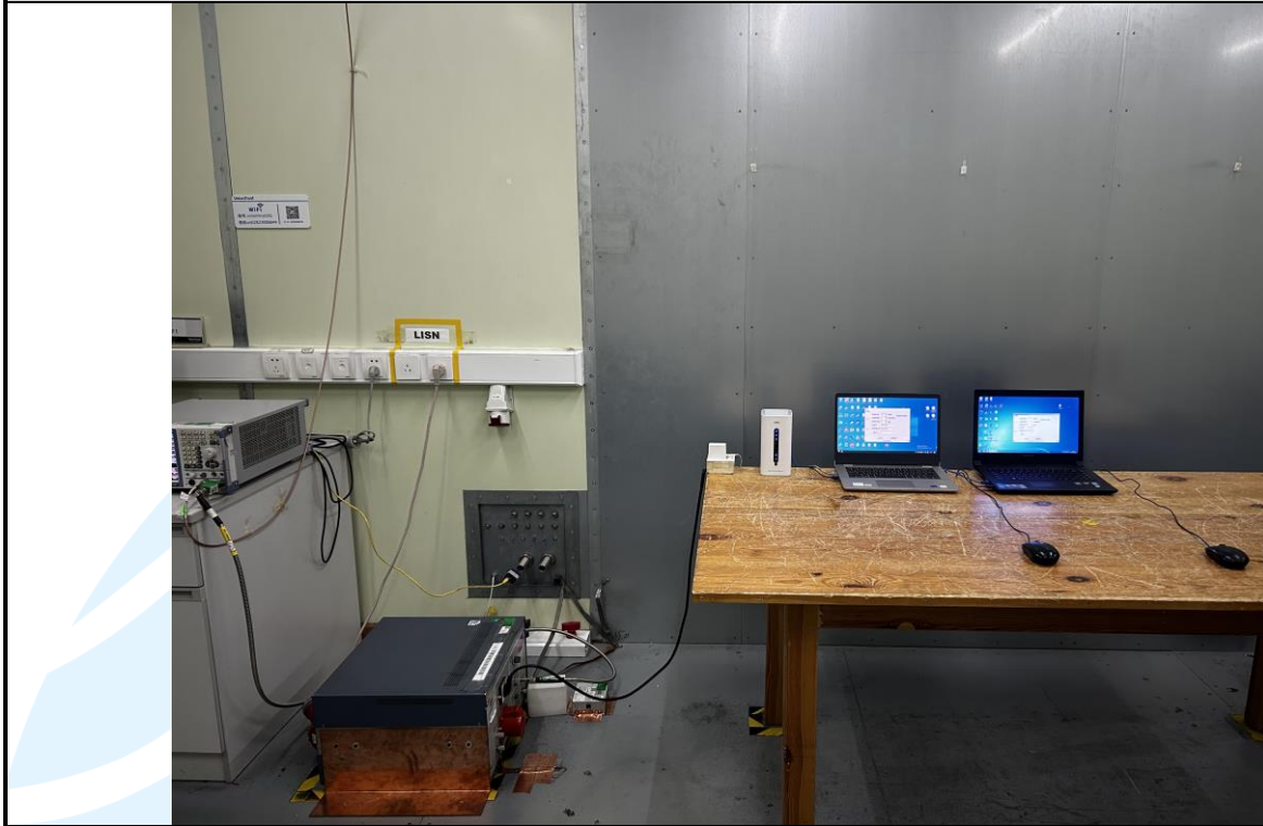
Conducted Emission Test Setup
