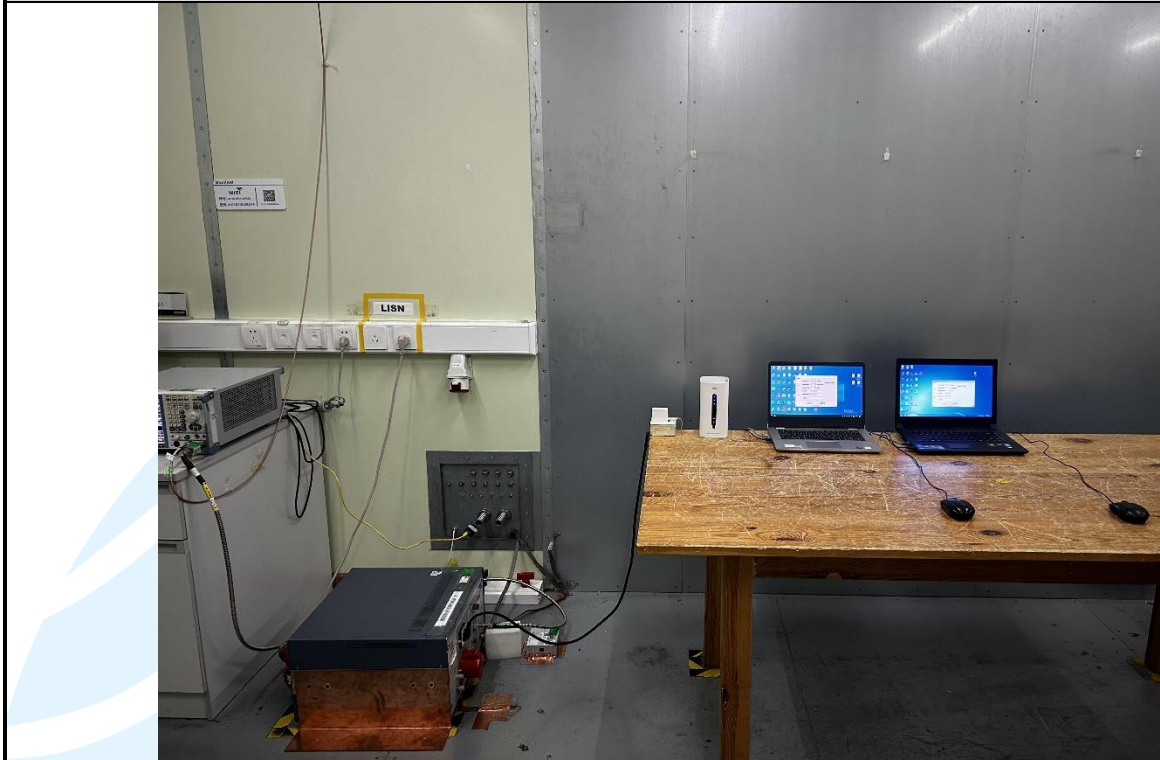
Conducted Emission Test Setup
