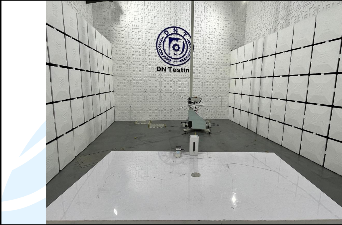
Radiated emission Test Setup (30 MHz~1 GHz)
