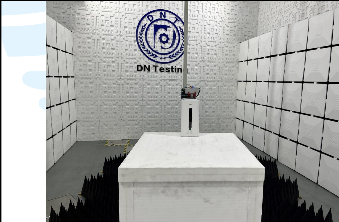
Radiated emission Test Setup (Above 1 GHz)
