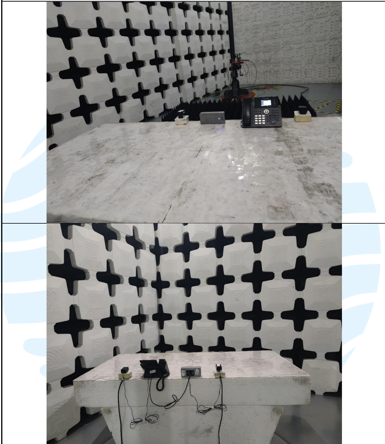
Radiated emission Test Setup-2 (Above 1 GHz)
