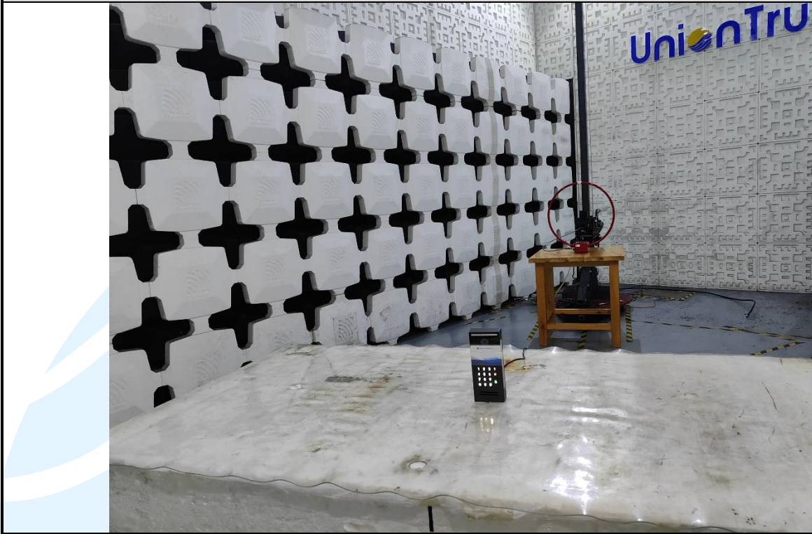
Radiated emission Test Setup (below 30 MHz)
