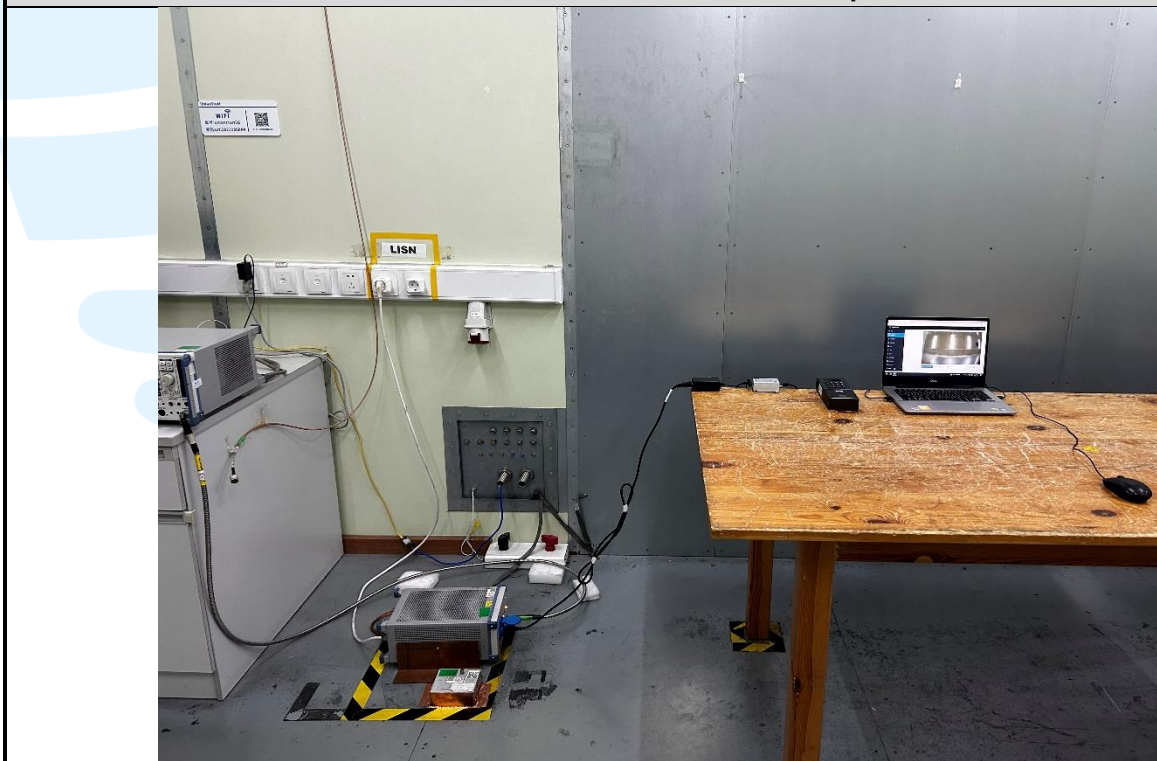
Conducted Emission Test Setup
