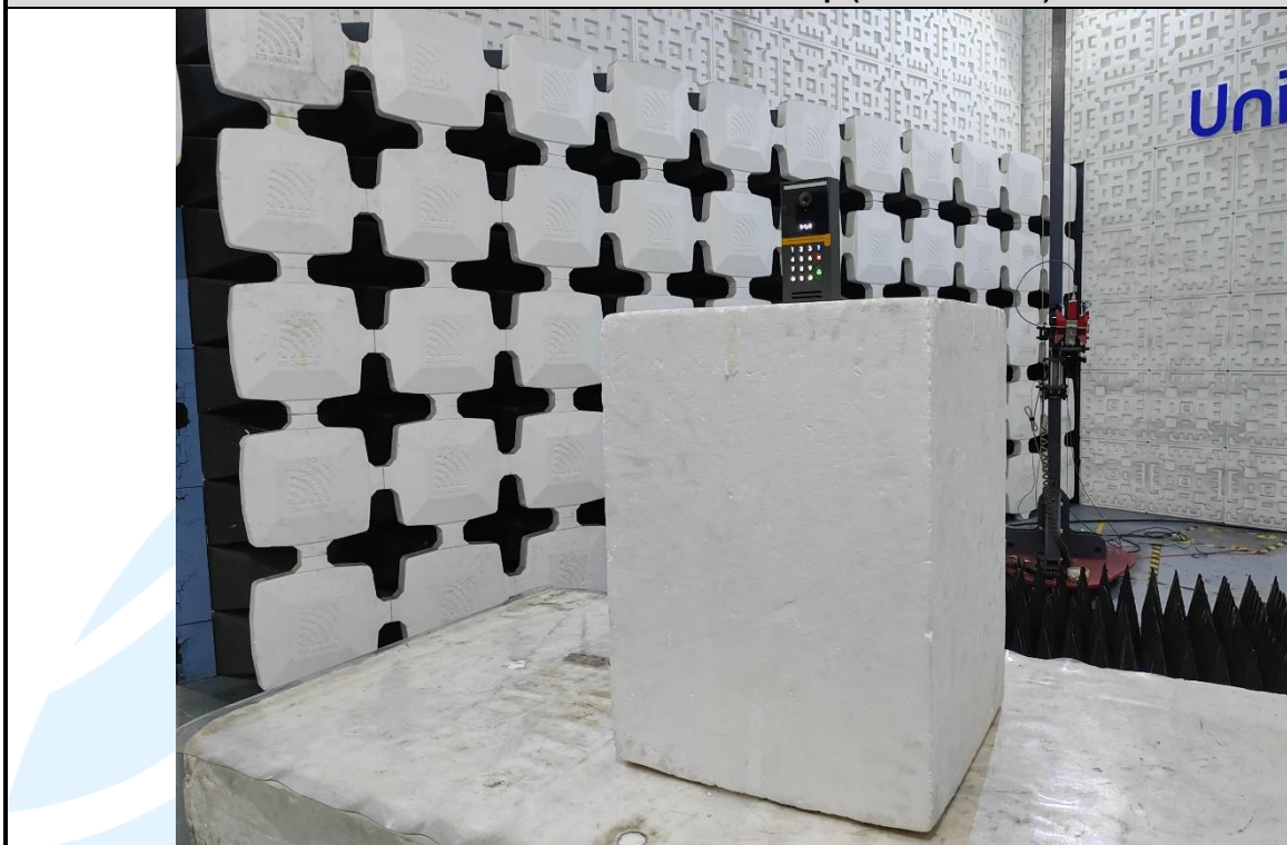
Radiated emission Test Setup (Above 1 GHz)
