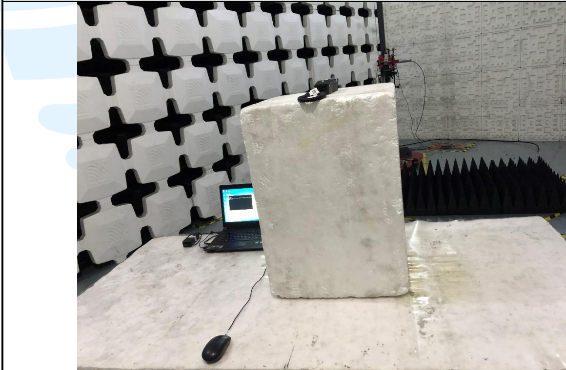
Radiated emission Test Setup (Above 1 GHz)
