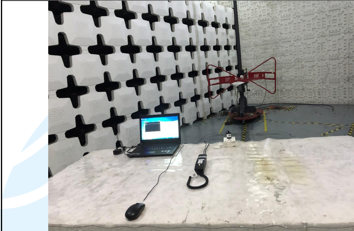
Radiated emission Test Setup (30 MHz~1 GHz)
