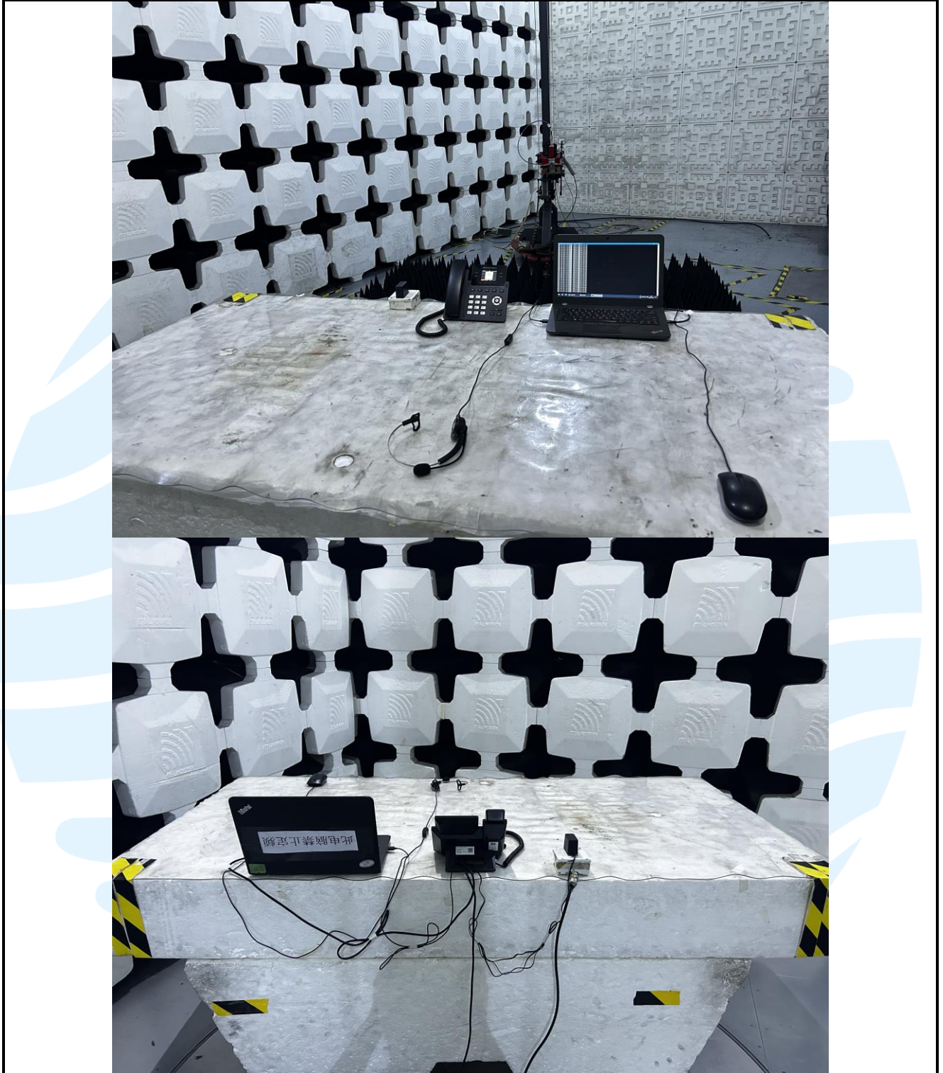
Radiated emission Test Setup-2 (Above 1 GHz)
