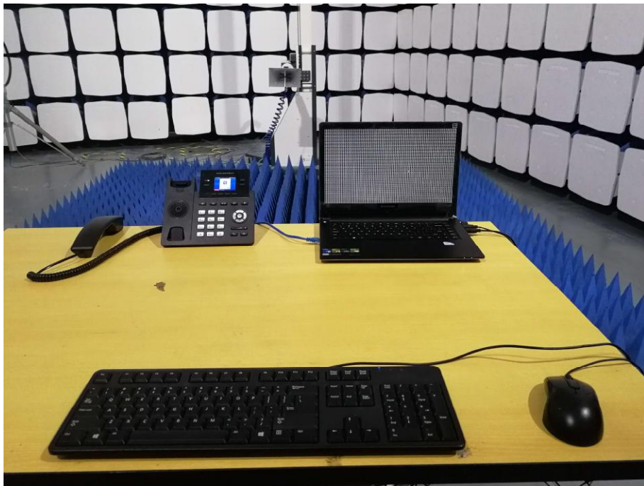
Radiated Emission test view (Above 1GHz)
