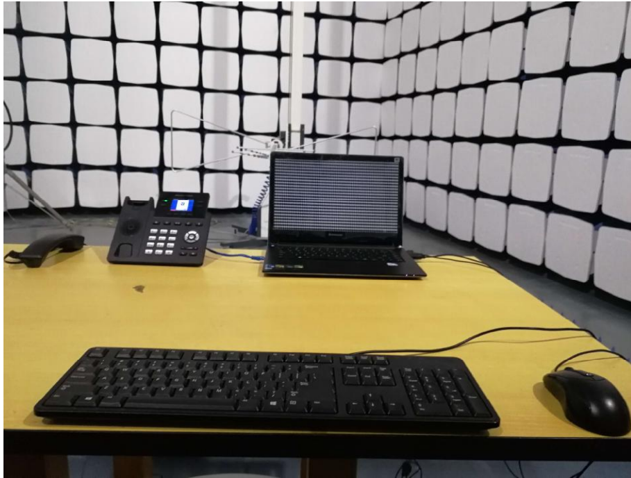
Radiated Emission test view (Below 1GHz)
