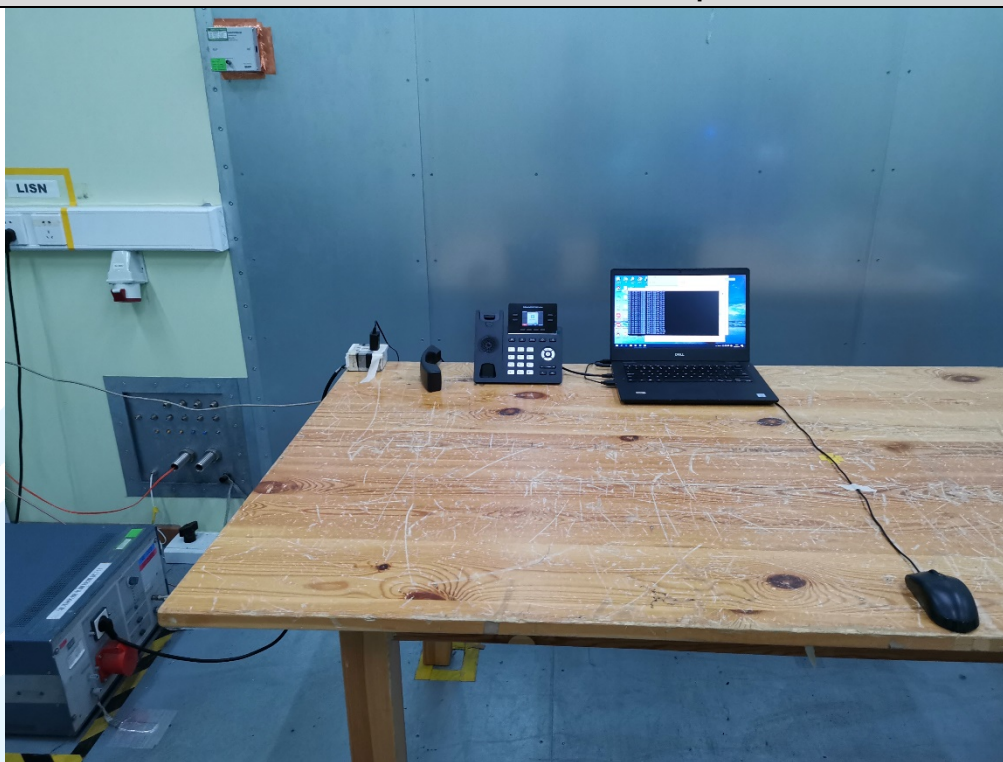
Conducted Emission Test Setup
