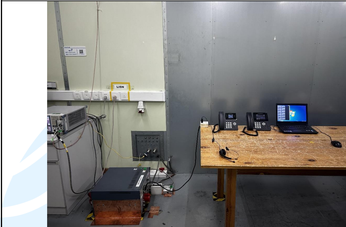
Conducted Emission Test Setup
