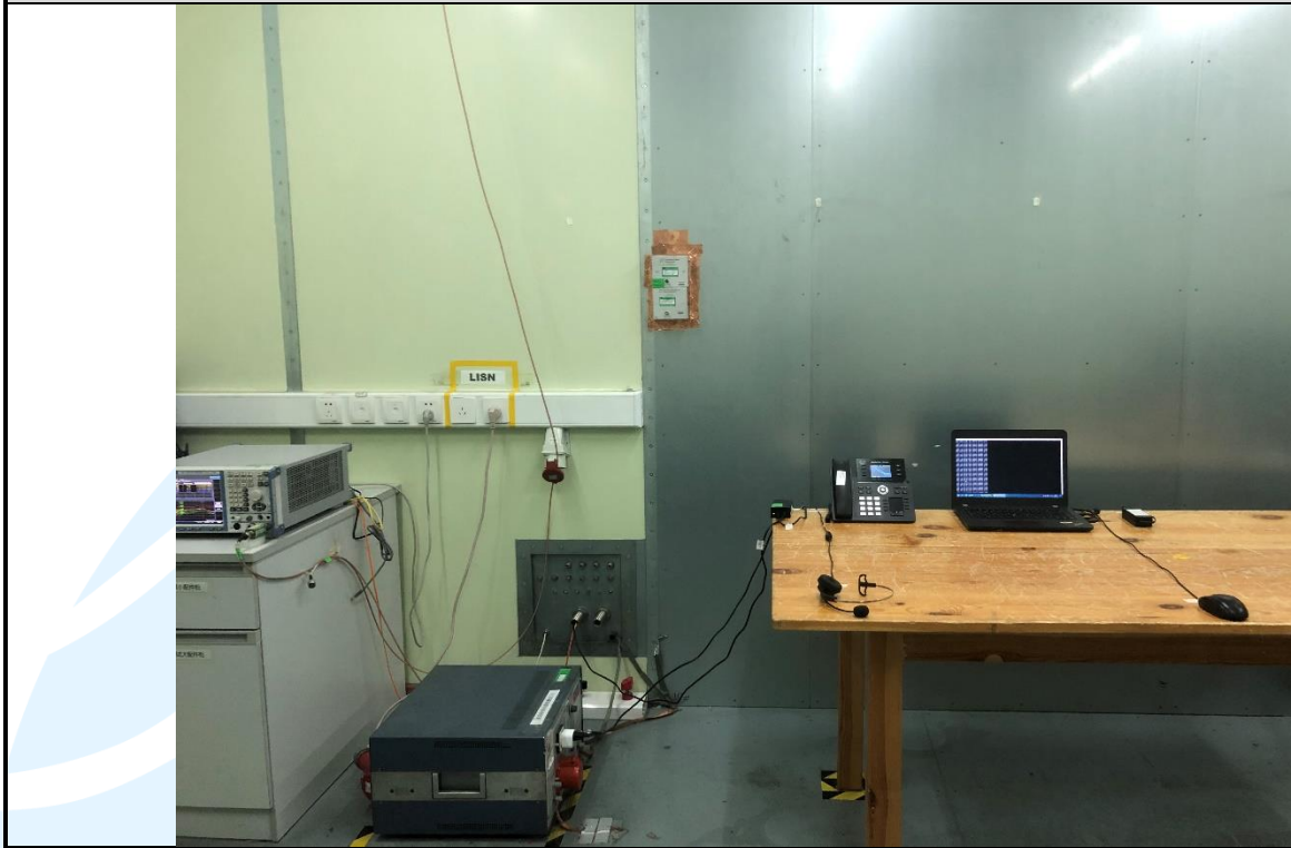
Conducted Emission Test Setup
