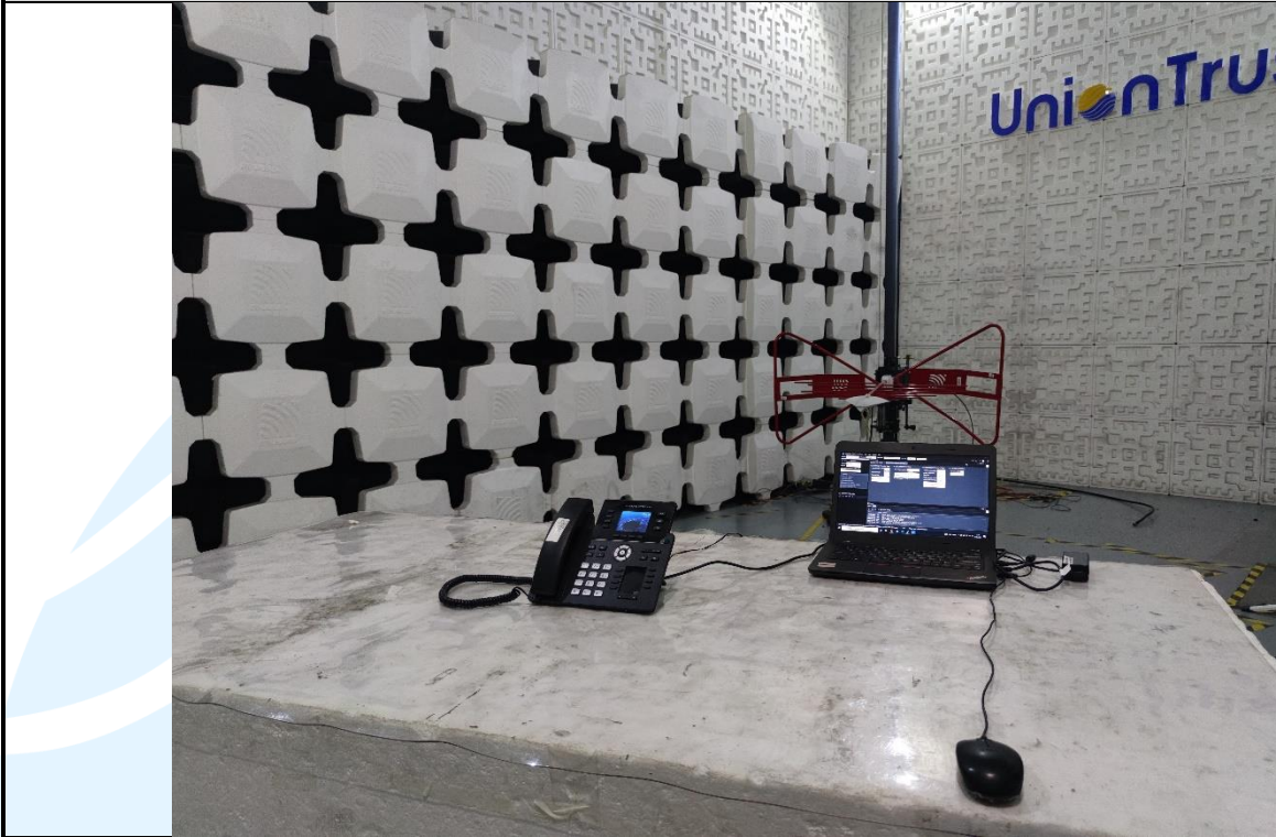
Radiated emission Test Setup (30 MHz~1 GHz)
