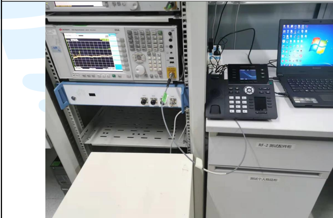
RF Conducted Test Setup
