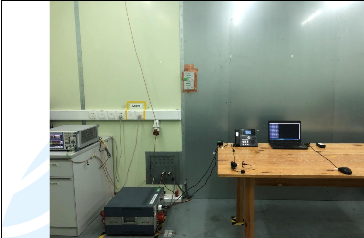
Conducted Emission Test Setup
