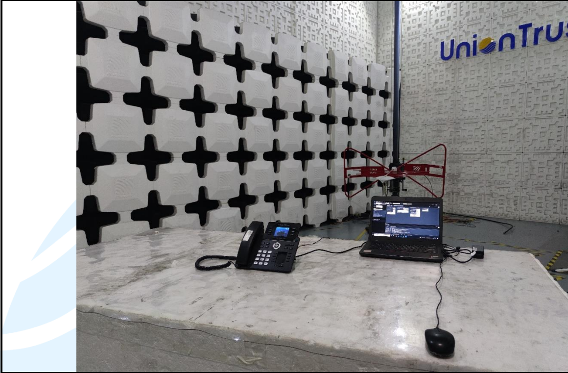
Radiated emission Test Setup (30 MHz~1 GHz)
