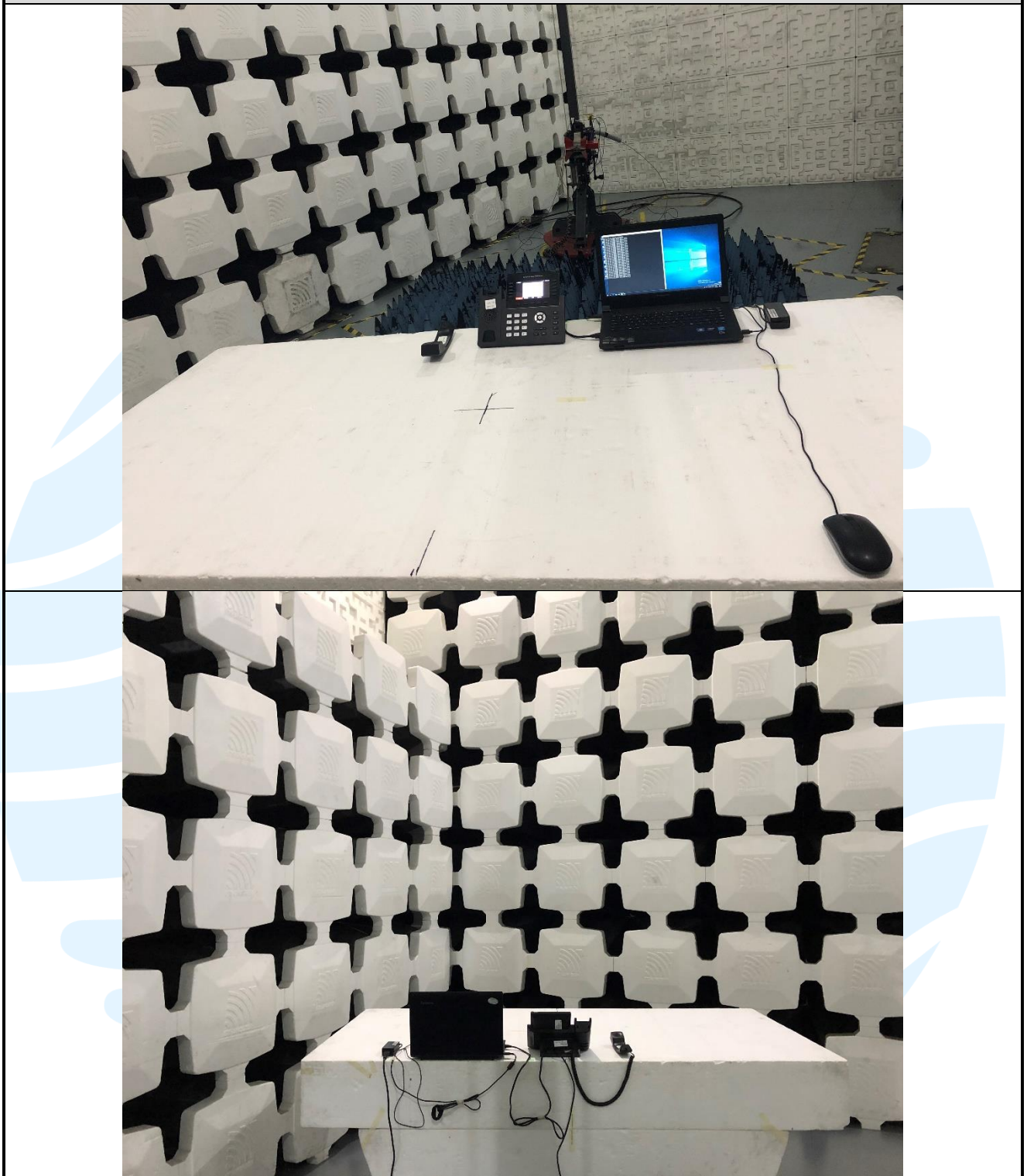
Radiated emission Test Setup (Above 1 GHz)
