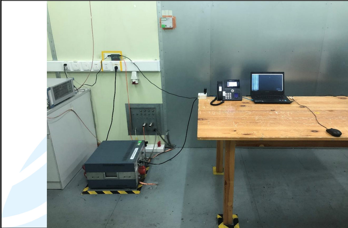
Conducted Emission Test Setup
