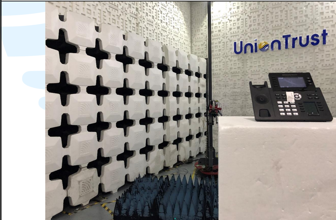
Radiated emission Test Setup (Above 1 GHz)
