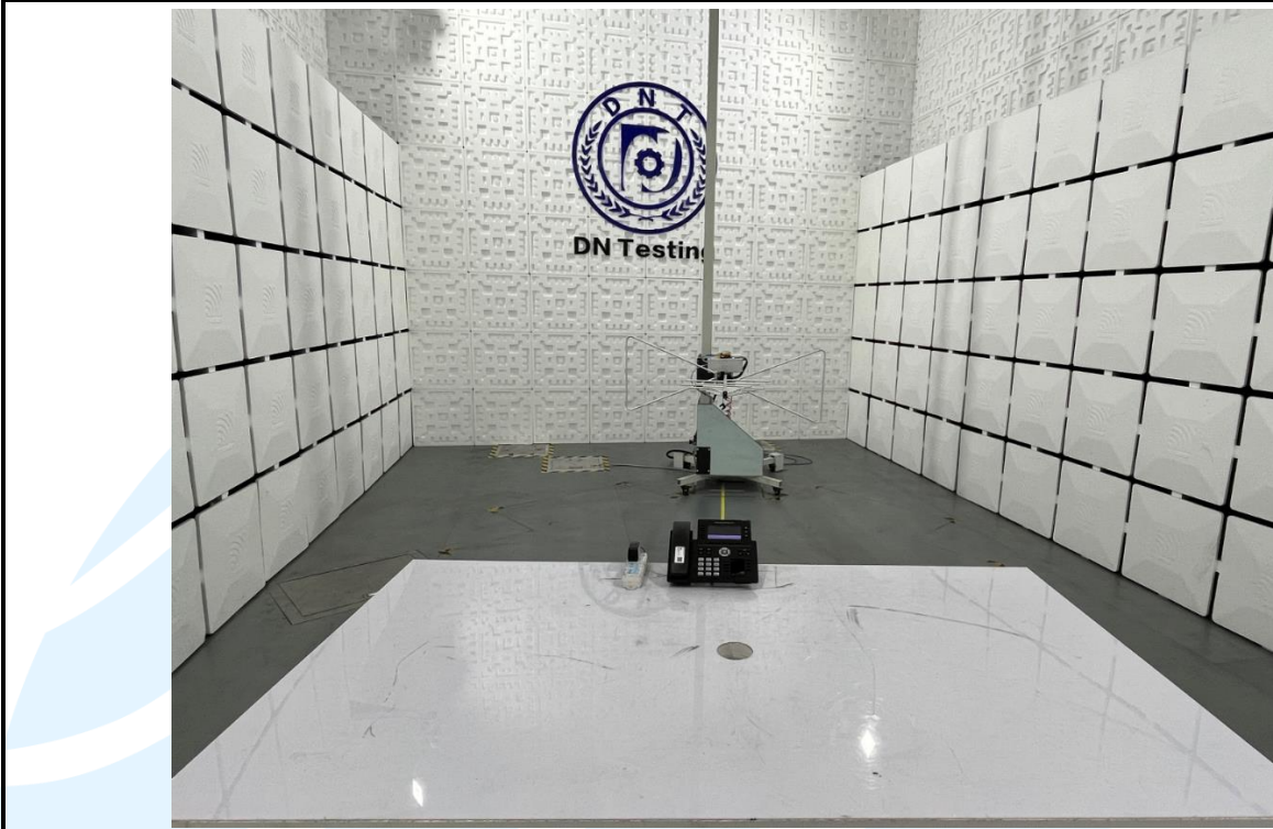
Radiated emission Test Setup (30 MHz~1 GHz)
