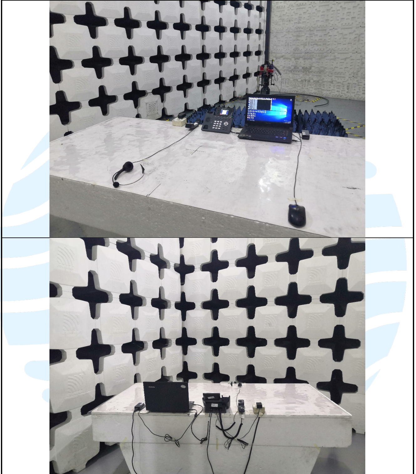
Radiated emission Test Setup-2 (Above 1 GHz)
