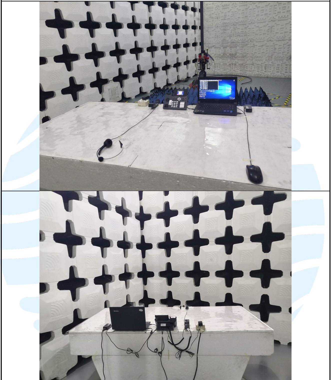
Radiated emission Test Setup-2 (Above 1 GHz)
