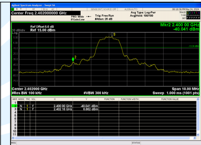
Out Of Band Emission \pi /4DQPSK_2-DH5_Channel 0
