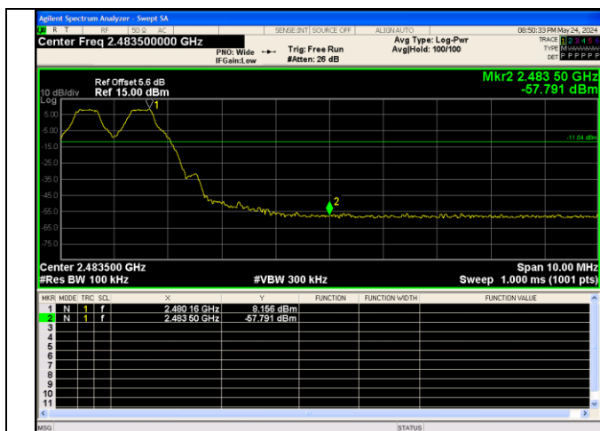
Out Of Band Emission(Right) GFSK_DH5_Channel Hopping
