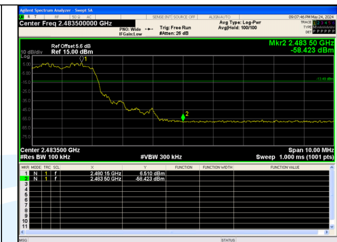
Out Of Band Emission(Right) \pi/4 DQPSK_2-DH5_Channel Hopping
