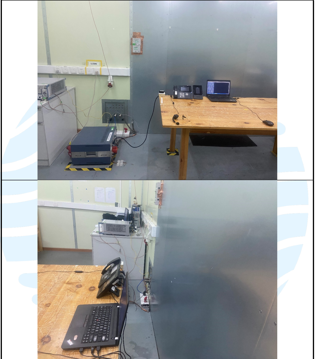
Conducted Emission (AC Port) Test Setup-5
