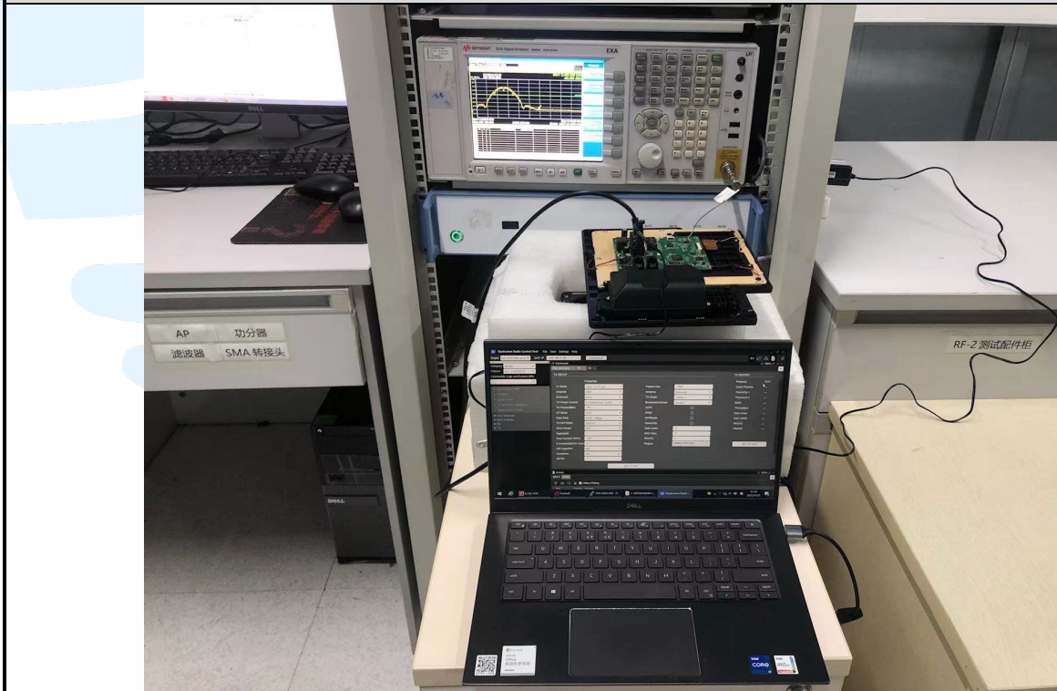
RF Conducted Test Setup
