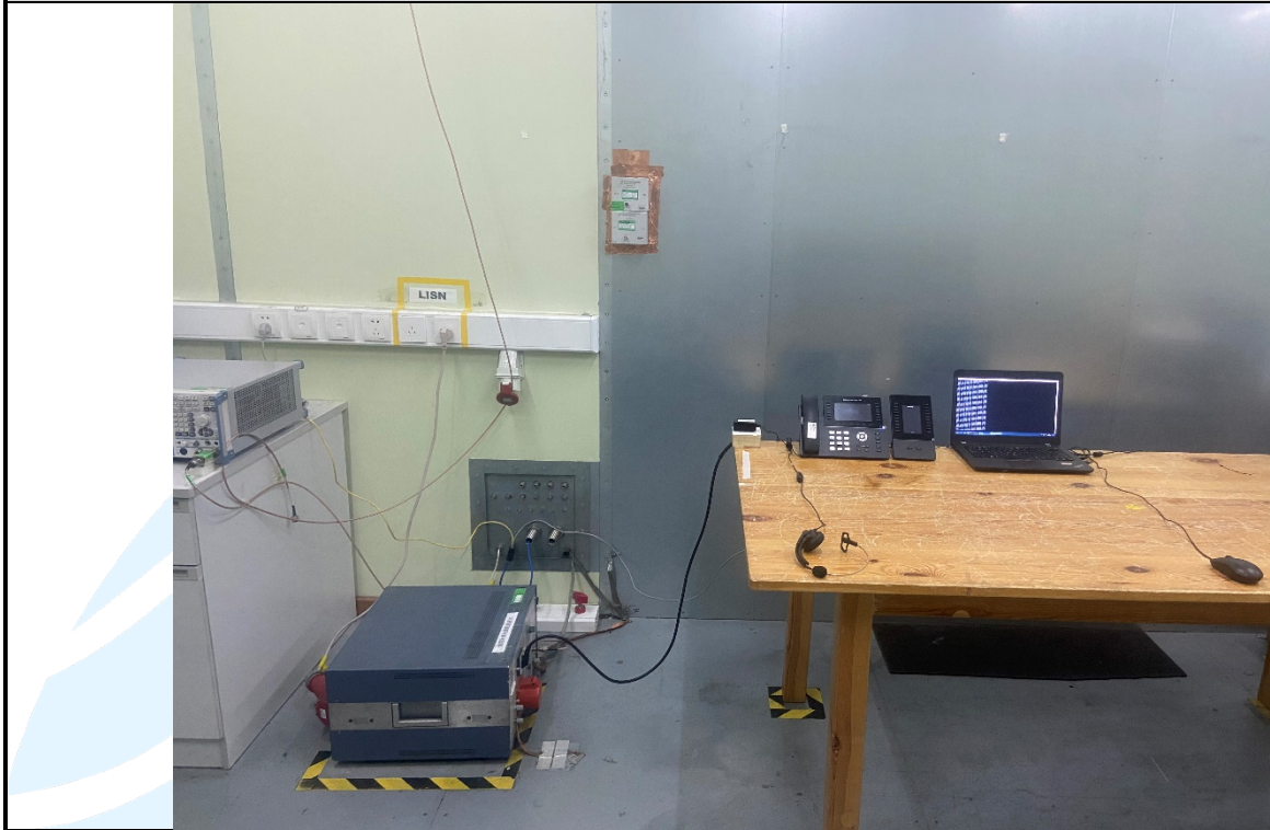
Conducted Emission Test Setup
