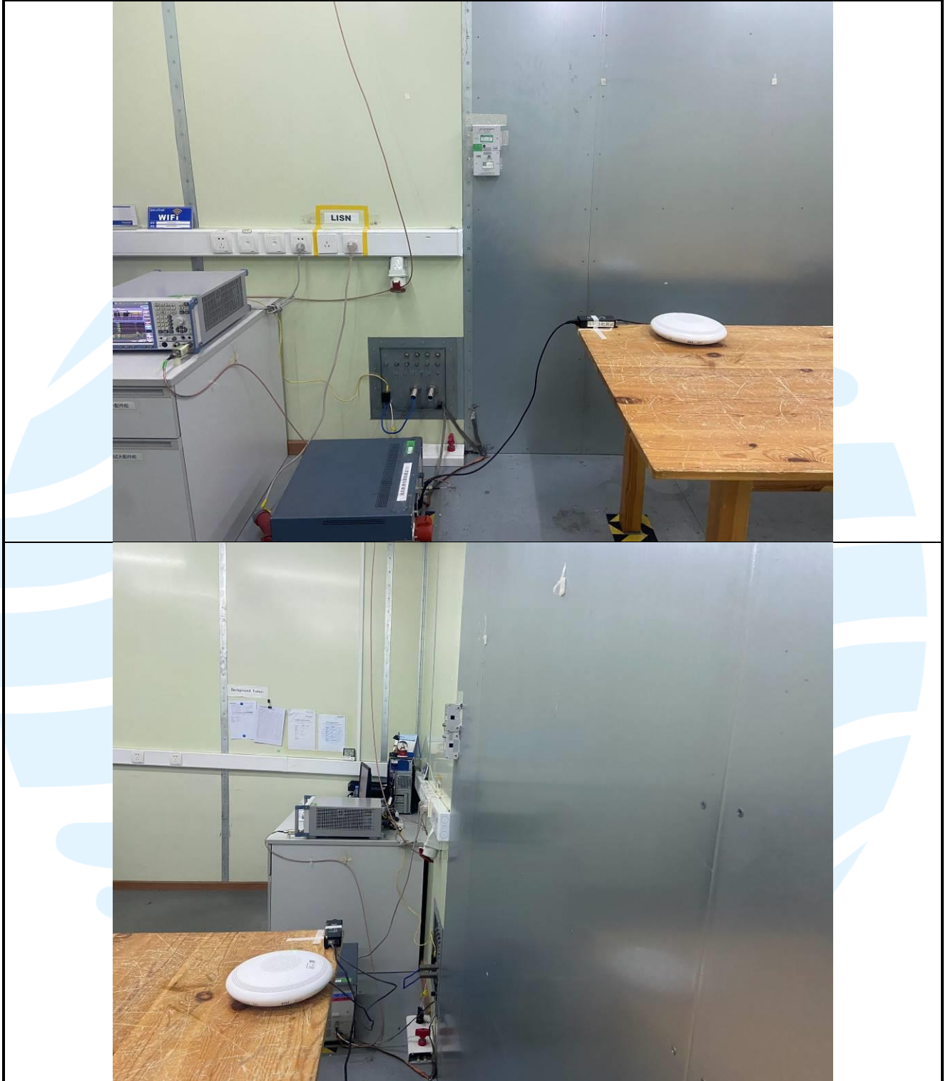
Conducted Emission Test Setup-3
