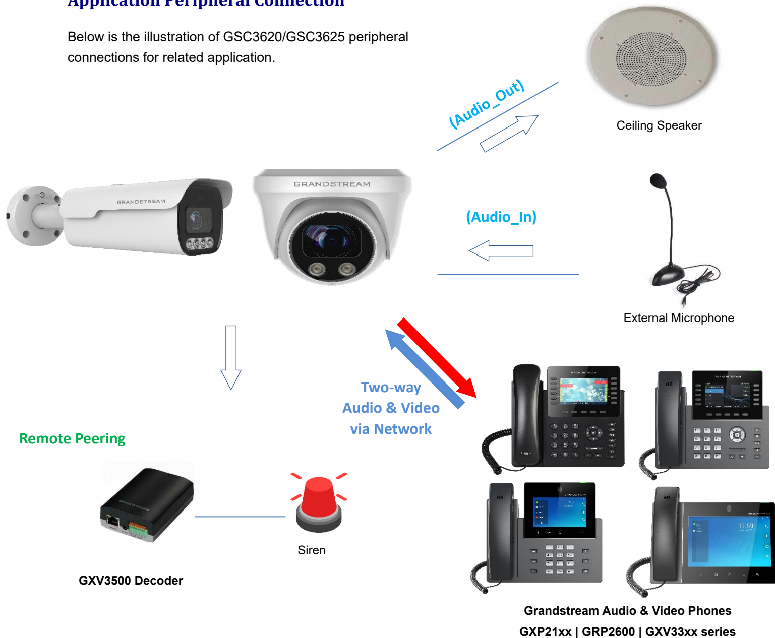
Figure 8: Application Peripheral Connection for GSC3620/GSC3625
