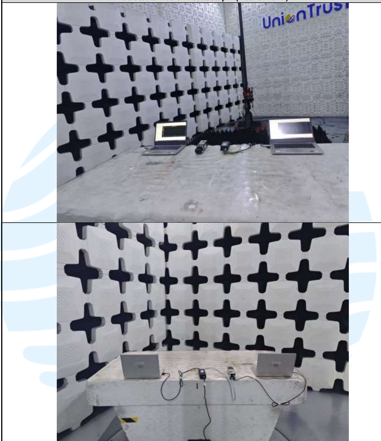
Radiated emission Test Setup-2 (Above 1 GHz)
